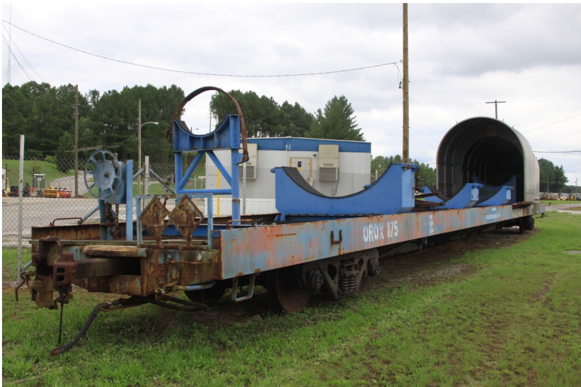
The flat bed railroad car modified to transport the Navy's submarine to the test site
